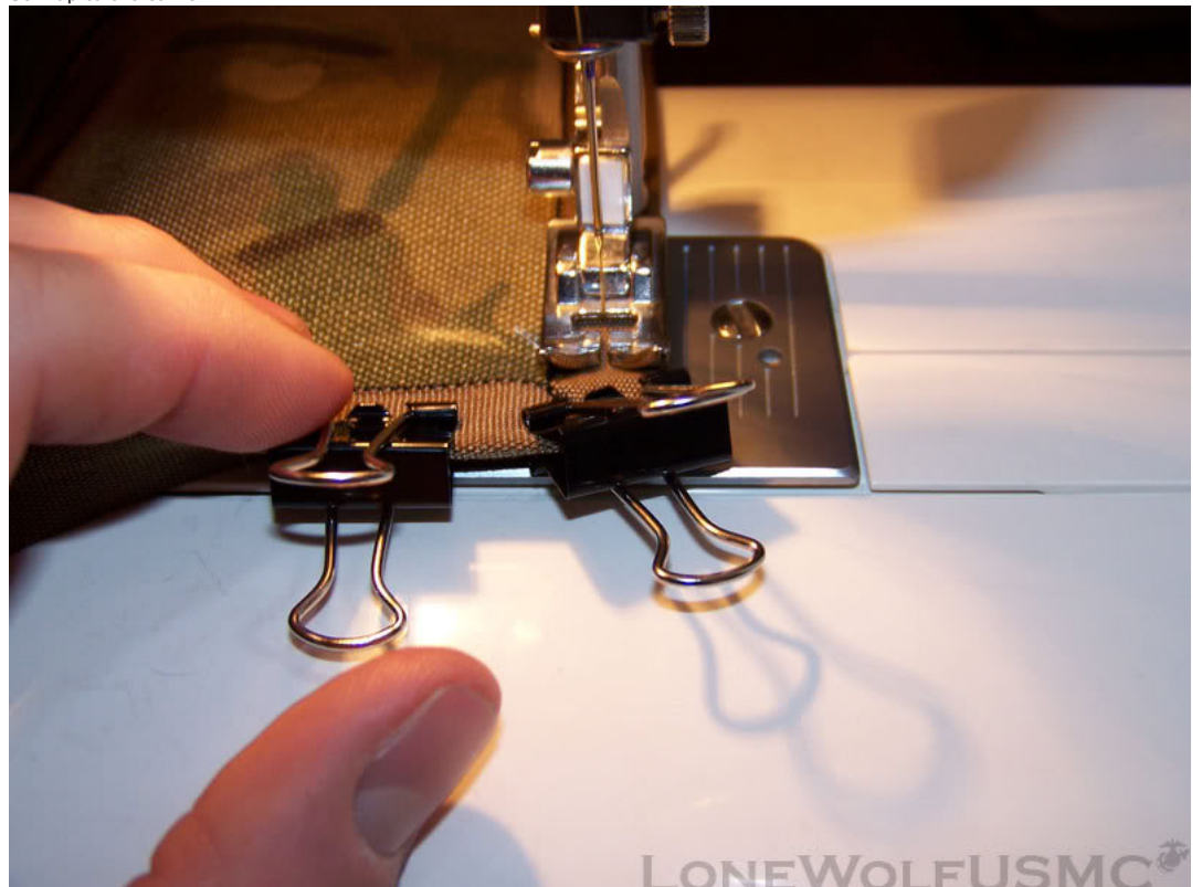
Remove the clip when the presser foot is close enough to hold the fold.
