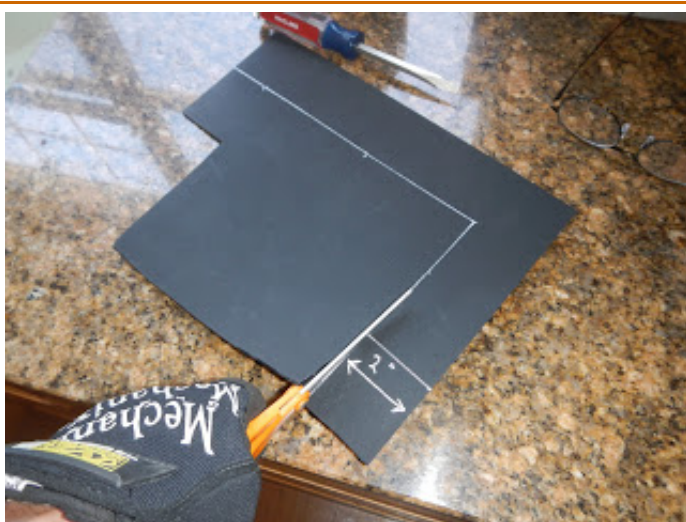
Cutting the Kydex with scissors
