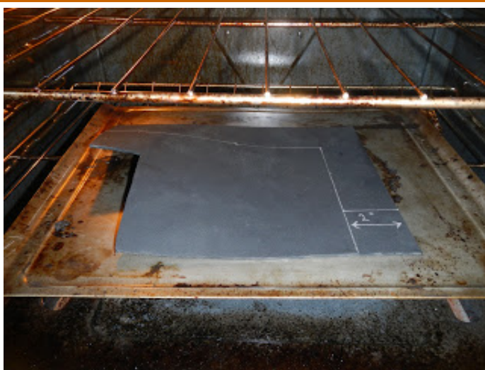
Put the Kydex in the oven and wait to soften up.
