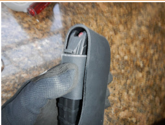
Forming Kydex around the magazine.
