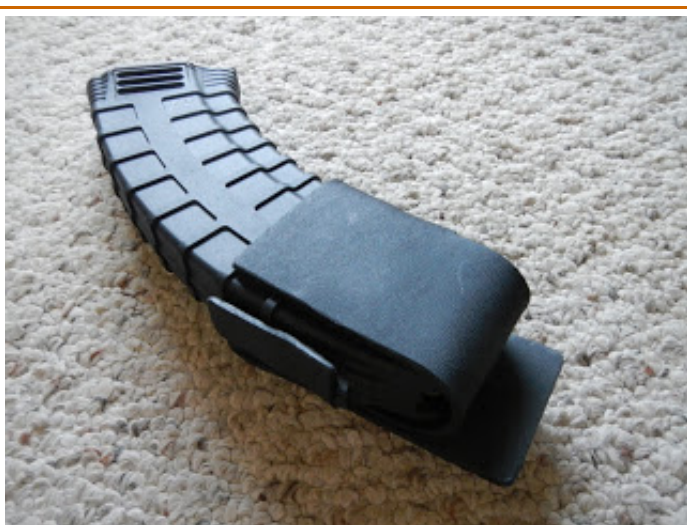
One piece of Kydex hand wrapped around magazine.
