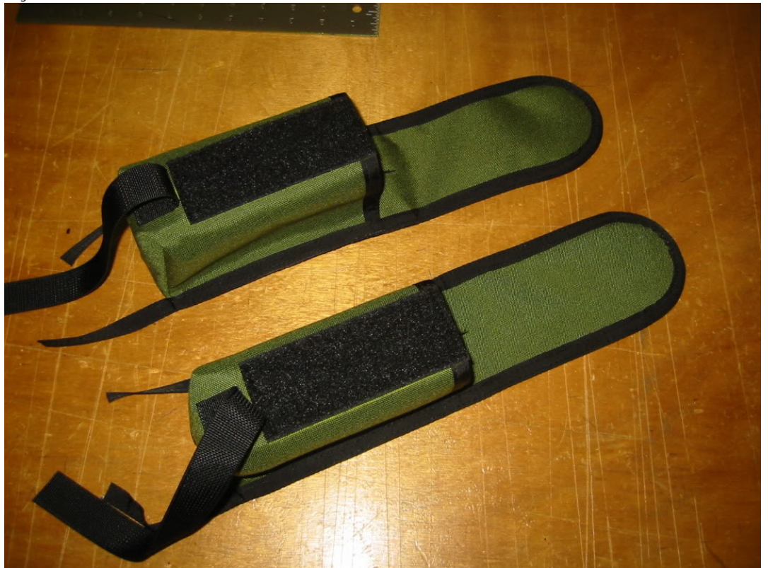
Cut your edge binding long enough to double fold.
