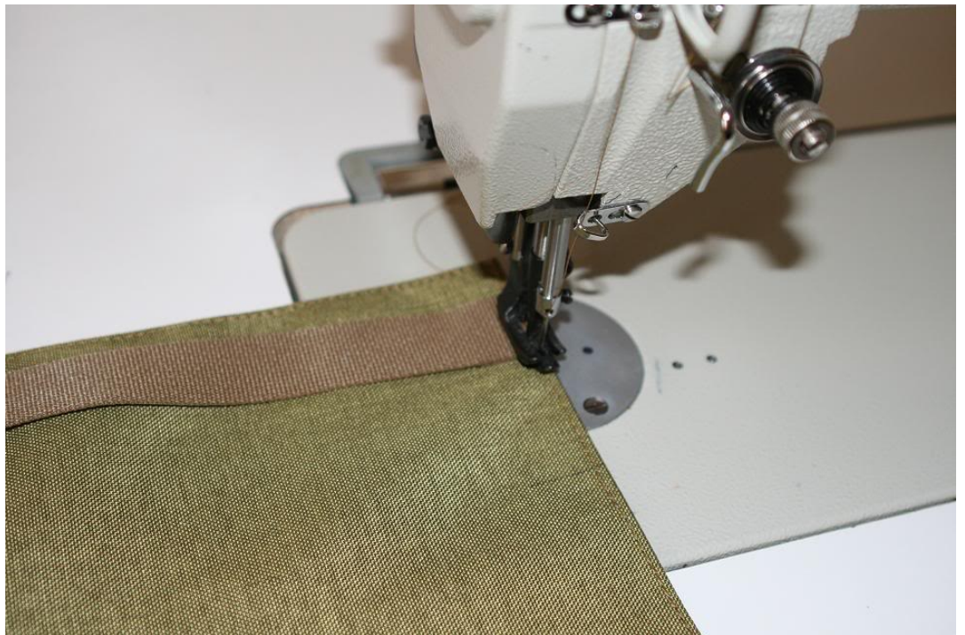
Laying out the webbing. I fold my ends in so I cut the strips to 29" long. Remember to fuse the ends.
